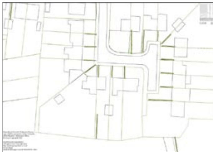
Figure 5. Radius Topology can show the user which BLPU boundaries do not completely line up with the Ordnance Survey mapping.
