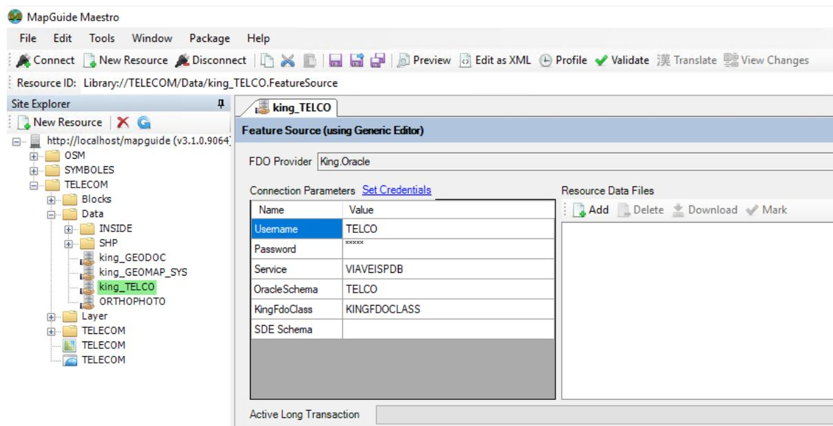
The Site Explorer panel shows a tree structure with categories like OSM, SYMBOLES, TELECOM, Data, SHP, and Layer. Under TELECOM, there are sub-folders like Blocks, INSIDE, and SHP, which contain tables like king\_GEODOC, king\_GEOMAP\_SYS, and King\_TELCO. The Feature Source (using Generic Editor) panel displays connection parameters for a King.Oracle provider:
