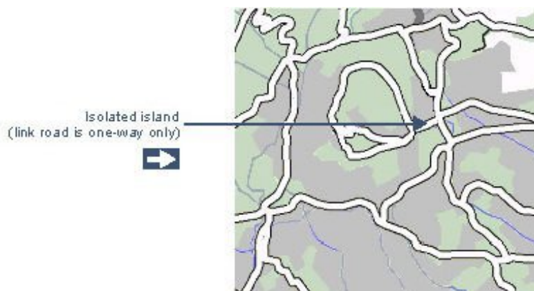
Figure 6-3: Isolated island (restricted access to network)
