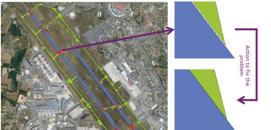
Figure 2: violation of rule 6 of ED-99c and corrective action
